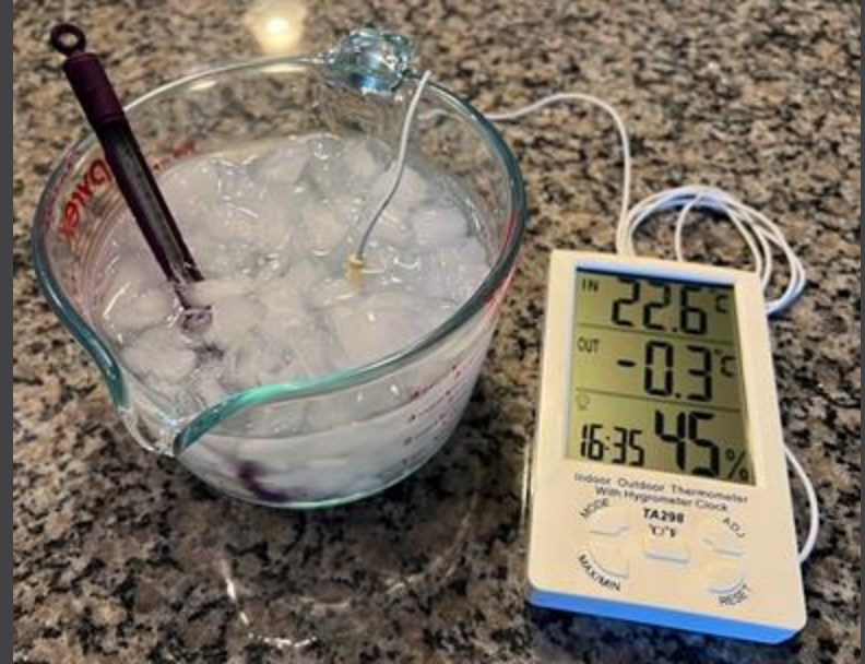
Testing the calibration of a liquid filled thermometer and a digital thermometer at the same time. Credit: GLOBE
